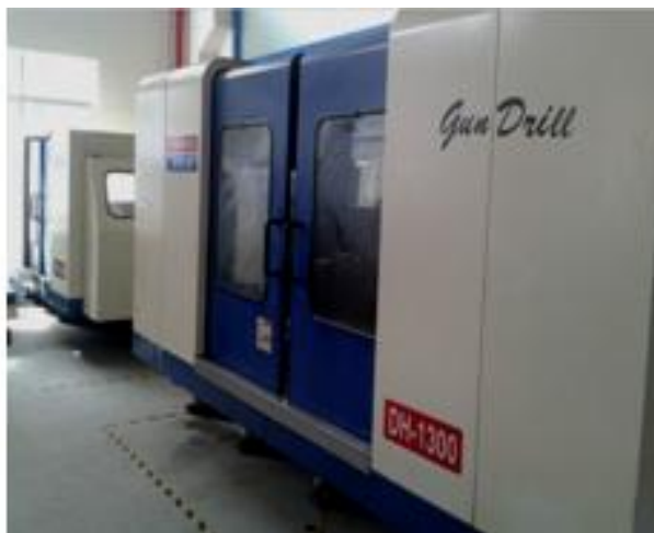
1.3M Deep Hole Drilling
