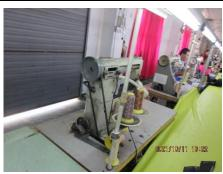
No. 1: The sewing machine was missing belt pulley safety guard in 3/F stitching workshop
